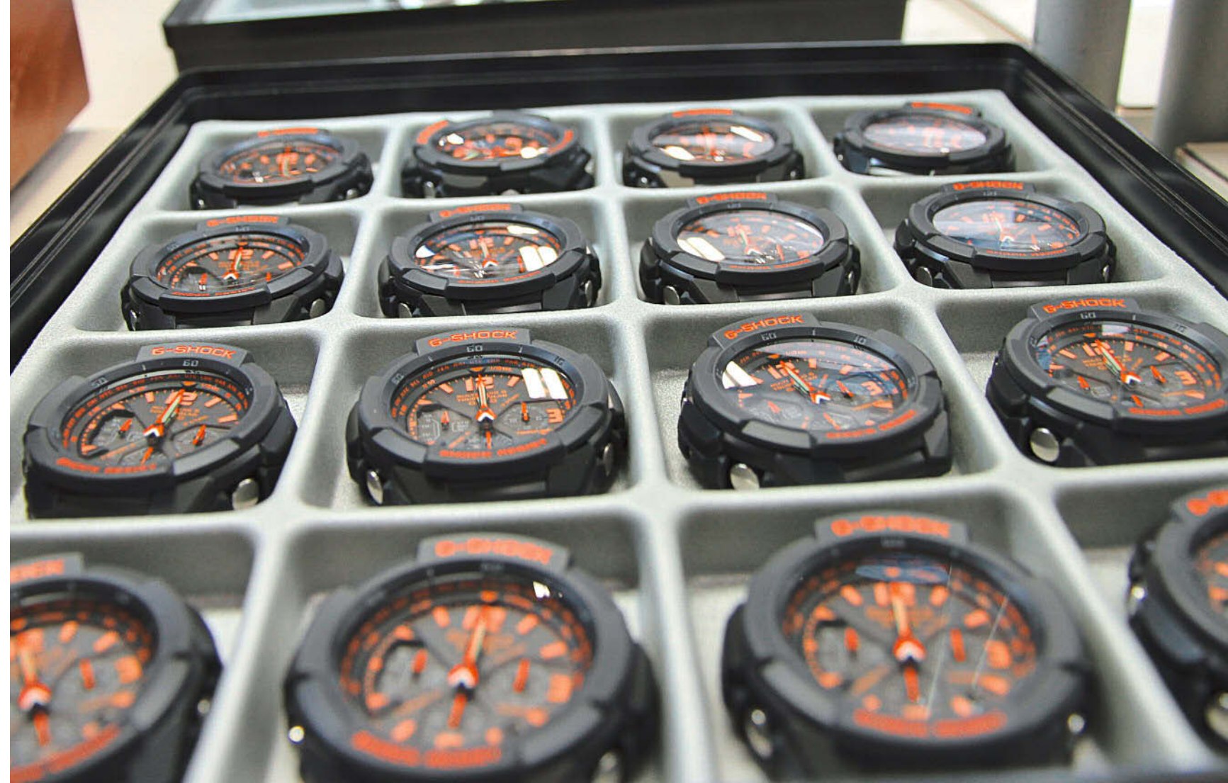
A tray of G-Shock Aviation watches being prepared for water-pressure testing
